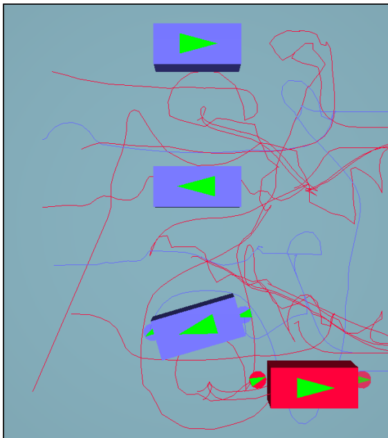
Figure 80: Movement near end of simulation. Notice that the red occupants needing assistance have been helped. Two blue beds are still waiting for assistance, since there are only two members in the blue team it takes longer to assist the blue occupants.
